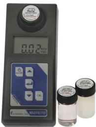
Designed to provide the ease of portability needed in the field with rugged durability, the MicroTPW is a necessity for anyone monitoring turbidity on the go. The shock-resistant carrying case holds everything necessary for field operation while the instrument itself removes easily to go wherever it is needed.
