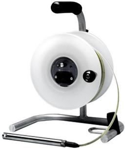
The Geotech ET and ETL Portable Water Level Meters are designed to provide reliable and accurate measurements of groundwater levels. Water level readings are taken at the top of the casing.
