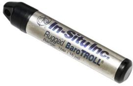
The BaroTROLL Data Logger measures and logs barometric pressure and temperature, data needed to compensate for water level changes due to barometric fluctuations. Use this data logger with non-vented (absolute) Aqua TROLL 100/200 or Level TROLL 400/700 water level loggers.
