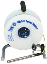
Provides reliable and accurate measurements of groundwater levels. Water level readings are taken at the top of the casing. They utilize a durable polypropylene storage reel with a rugged solid aluminum frame. Their highly accurate Polyethylene-coated steel tape.
