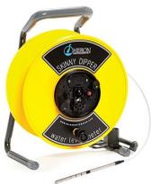
The SKINNY DIPPER water level meter is ideal for measuring static water levels in narrow wells, boreholes, tubes and piezometers. The slim line tape and 1/4" probe enable users to take readings while the pump is still in the well, whereas wider tapes may get tangled.
