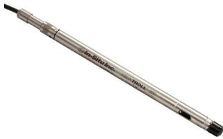
The In-Situ Aqua TROLL 200 instrument simultaneously measures and logs water level, conductivity and temperature. Features 4-electrode conductivity cell is less subject to fouling and resists electrical field effects from pumps and well casings.
