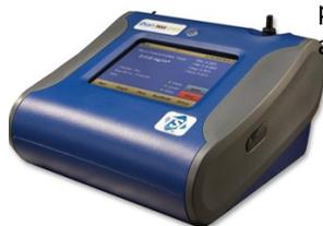
The DustTrak™ II Aerosol Monitor 8530 is a desktop battery-operated, data-logging, light-scattering laser photometer that gives you real-time aerosol mass readings. It uses a sheath air system that isolates the aerosol in the optics chamber to keep the optics clean for improved reliability and low maintenance.
